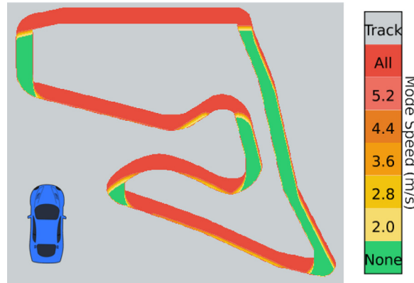
Fig. 7. The kernel for the AUT map for the vehicle facing the top of the map. The colours represent the allowed speed in m/s.
