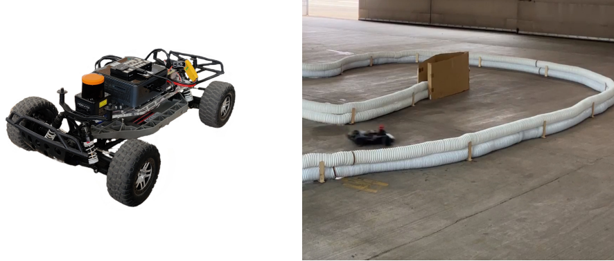
Figure 7. On the left, the physical F1TENTH system for Sim2Real RL deployment. On the right, a corner of the real testing track.
