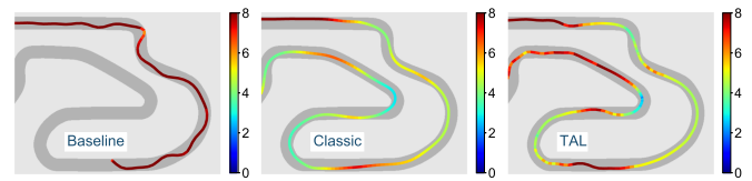
Fig. 14. Trajectories taken by the baseline (left), classical (middle), and TAL (right) agents on a portion of the ESP track.
